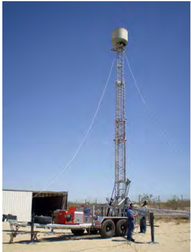
An LSTAR radar at the NUAIR UAS test site, in Rome, part of the site’s range instrumentation system providing real-time position data for inbound and outbound UAS, will aid in conducting Beyond Visual Line of Site UAS flights. Photo courtesy of the NUAIR Alliance.
