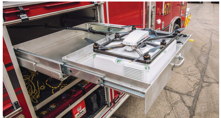
Fotokite Sigma is a vehicle-integrated aerial camera system that provides public safety teams with mission critical situational awareness.
